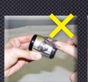
DO NOT grease pressed fit surfaces (eg. outer shell) or outside of shackles bushes. NOTE: The major noise producing factor in polyurethane is incorrect fitment and uncleaned mating surfaces.
