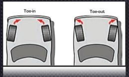
Toe describes how close to parallel the two tyres are, and whether they are toed-in (closer at the front of the tyre) or toed-out (closer at the rear of the tyre). The goal of toe is to provide proper tyre wear through various driving conditions. The amount of toe your suspension is set to varies by the drive layout of your vehicle, driving preference, and car's handling characteristics.
