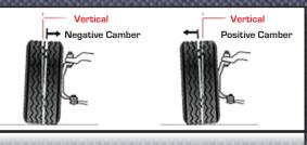
A tyre wears most at the point(s) where the majority of the vehicle's load rests. A properly set camber maximises a tyre's contact patch, leading to even wear. Excessive negative or positive camber has an adverse effect on treadlife by causing premature outer or inner shoulder wear.
